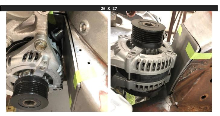
With the engine in position on the mounts the alternator should have clearance both to the side and behind to the frame. Once the position is finalized, the engine can be removed and the patch panel welded into place.
