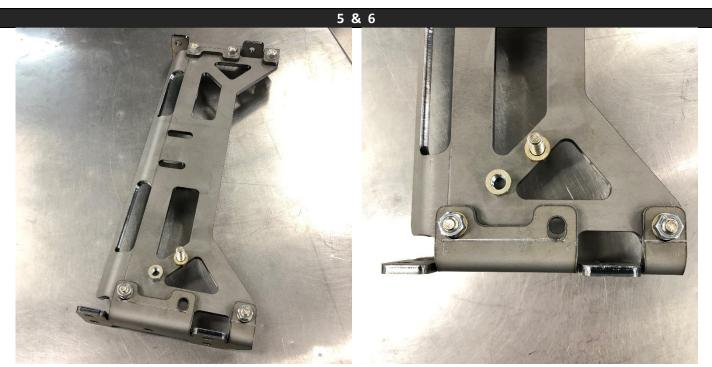
**For 6r80 and 10r80 transmissions, skip to Step 9.** For 4r70w transmissions, position the transmission crossmember so that the bent leg is towards the **front** of the car and **down**, and that the crossmember plate attaches **underneath** the L brackets at the sides, as shown (driver side is in the foreground of the photo). The six 3/8 connections to the crossmember allow for 2 bolting options: 61-65 cars will use the narrow configuration, whereas 66-69 will use the wide configuration.
