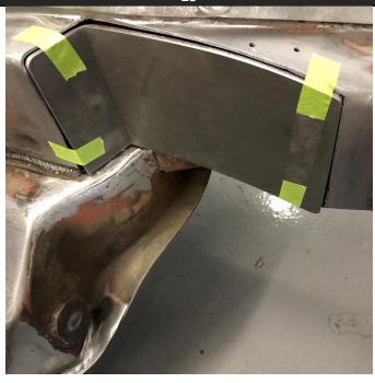
It is advised only to fit the patch panel at this time, while using a tack weld or tape to hold it in place for fitment with the engine and alternator to confirm it doesn't need to be shifted.
