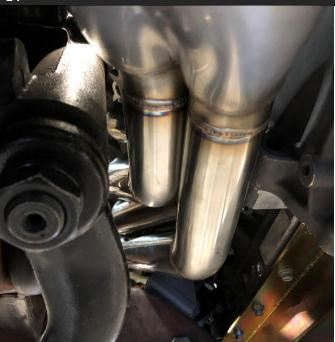
There are several clearance "hot spots" to contend with when using the Coyote engine in the Lincoln. The Lincoln steering box poses a major issue both to the driver side cylinder head and to any factory or aftermarket exhaust systems. It is recommended to use our <u>Lincoln / Coyote Swap - Headers</u> for this reason as they were designed to make the best use of space with these engines in these cars.
