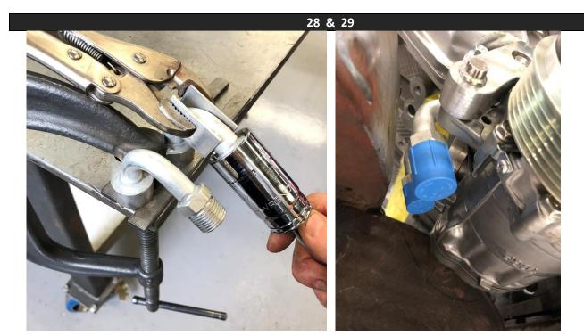
The Vintage Air Coyote Frontrunner (174020) can be used to add power steering functionality and AC. The <u>LSMFG Oil Pan</u> is also designed with a notch to be compatible with the tensioner included with the Frontrunner. The Vintage Air Tite-Fit Line kit (342310) can be lightly bent as shown using a socket along with support on each side to prevent distortion of the tubes.
