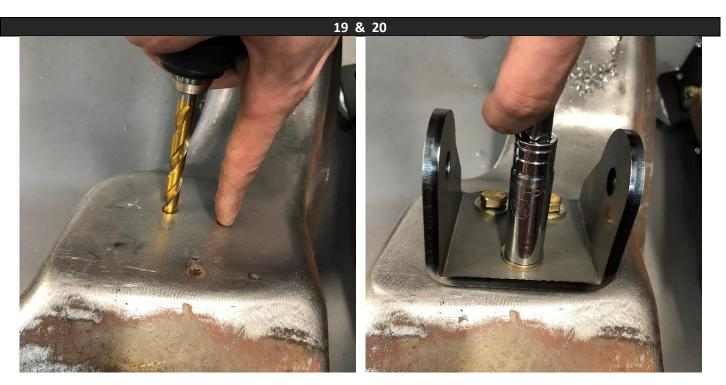
Step up to a 7/16 drill bit and finish drilling the holes in the crossmember. Then loosely install the saddles on the frame.
