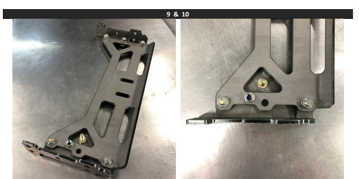
**For 4r70w transmissions, skip to Step 13.** For 6r80 and 10r80 transmissions, position the transmission crossmember so that the bent leg is towards the **rear** of the car and **up**, and make sure that the crossmember plate attaches **on top** of the L brackets as shown (driver side is in the foreground of the photo). The six 3/8 connections to the crossmember allow for 2 bolting options: 61-65 cars will use the narrow configuration, whereas 66-69 will use the wide configuration.
