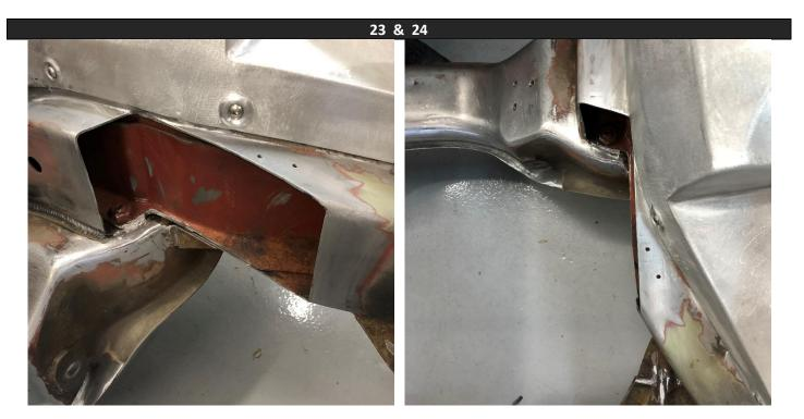
The cut will fit the patch part and look similar to what is shown, with the long leg of the "L" parallel to the centerline of the car.
