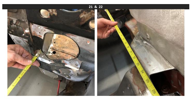
A frame patch is included to be used with Ford alternators such as **M-8600-M50BALT**. It can be installed by measuring from the location on the firewall as shown, marking for the rear edge of the notch to be cut at 24.875"
