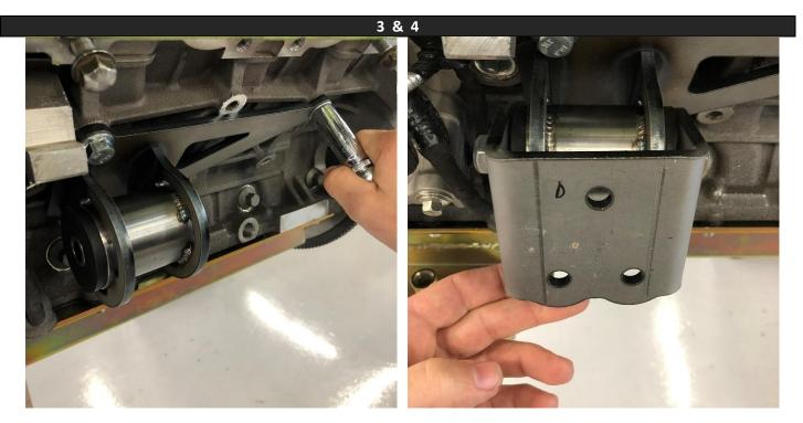
The engine mounts will bolt to the engine using three M10x1.5 x 25mm bolts on each side. The driver side is shown here and passenger is a mirror image. Bolt on the receiver saddle at this time using the supplied  $\frac{1}{2}$ -20 bolts, washers, and nuts. Position it so the 2 bolt holes are on the bottom as shown. Do not tighten completely at this time.
